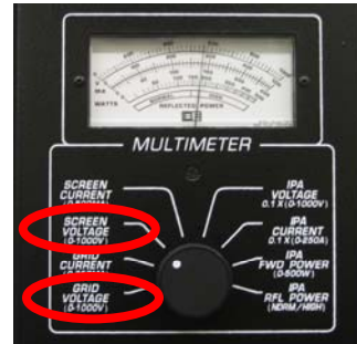
Figure 12 – Check Plate Voltage, PA Control Grid, and PA Screen Voltages
