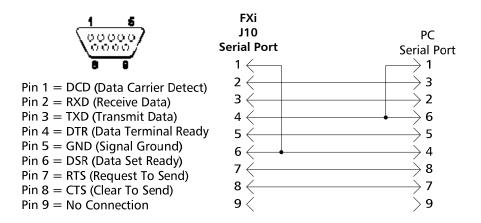
Figure 2 – Null Modem Cable Pinout
