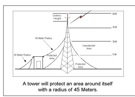
Lightning will strike the tallest conducting object in the vicinity. Thus a tall tower will shield the area surrounding the tower, and this area has the shape of a cone with the tower at its apex. The taller the tower, the larger the area that it shields.
