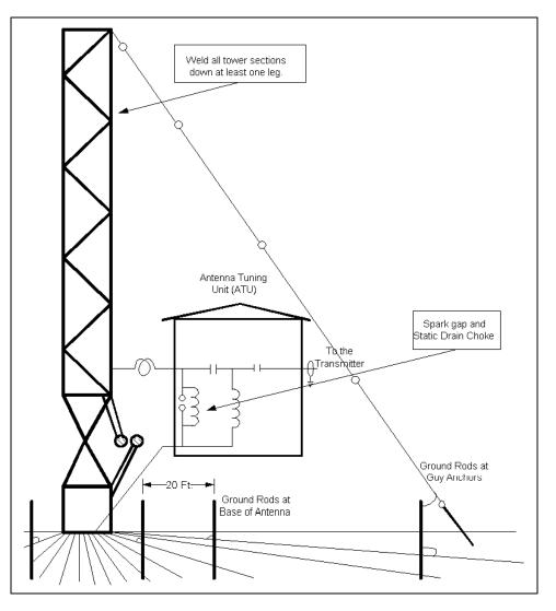
per 1,000 volts peak. Orient the terminals horizontally to keep rainwater out of the gap, and to assure that the gap is self-quenching. Periodically clean any corrosion from the spark balls, which would otherwise increase the resistance of the gap.
