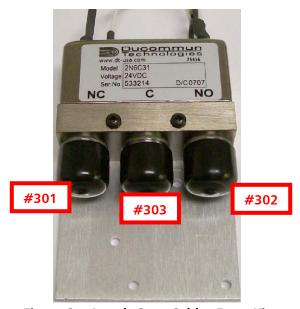
Figure 3 – Attach Coax Cables From Kit
