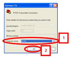
Figure 15 – HyperTerminal Connect To Menu
