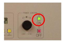
Figure 20 - Turn Transmitter's RF Output ON
