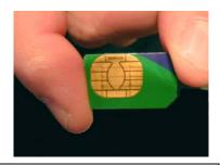
1)Typical SIM Card. This is the side that must face the PCB when you insert it in the Digital Cellcast.
