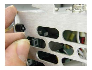
Adjust gap by screwing shaft in block until pin gage passes through with very little resistance.
