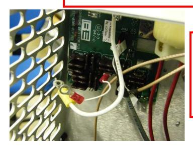
Use 3/8" wrench and Phillips screwdriver to remove hardware attaching wires to cap of glass tube spark gap.
