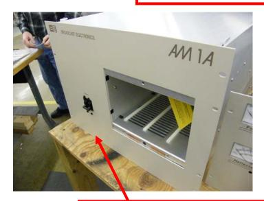
Install output network box in rack if necessary.
