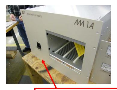
Remove output network box from rack if necessary.
