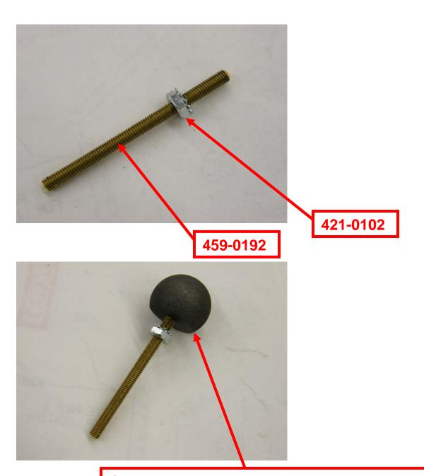
CAREFULLY screw shaft into 459-0189 until it bottoms. Make sure that the screw is square with the flat on the ball when you first engage threads. The first few threads are very delicate and can be easily broken if the screw is cross-threaded.
