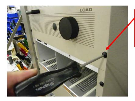
Remove and save the four screws on the front of the output network.
