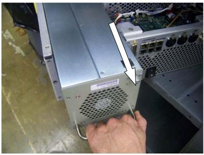
Figure 4. Remove power supply
