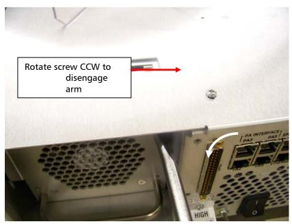
Figure 3. Disengage power supply
