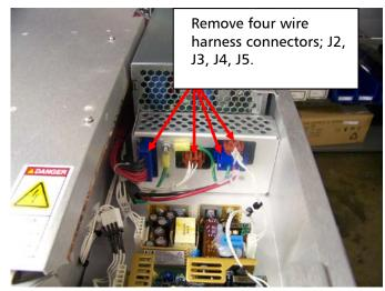
Figure 5. Disconnect wire harness
