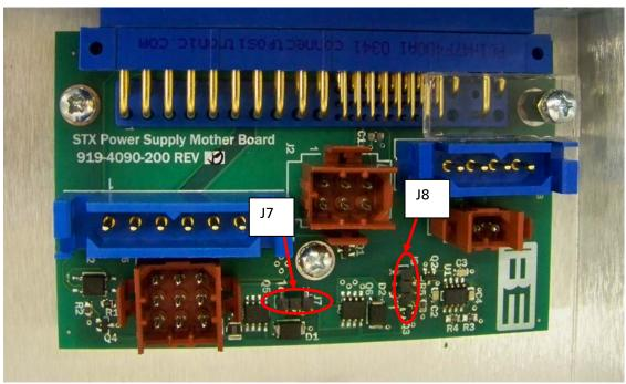
Figure 11. Fan speed selection if desired.
