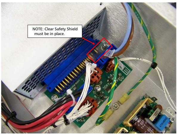
Figure 10. Power Supply Mother Board installed in chassis.
