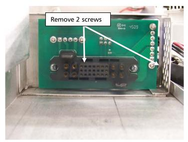
Figure 6. Remove mother board screws
