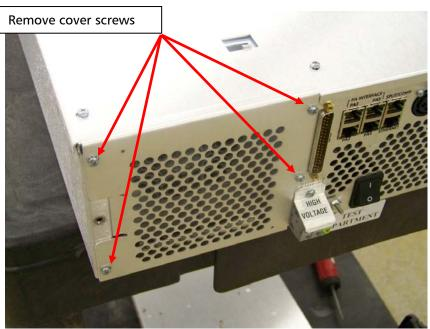
Figure 1.Remove Power Supply rear cover
