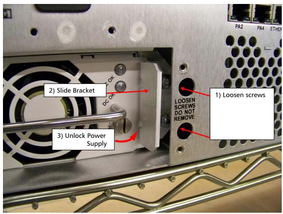
Figure 8.Remove Power Supply rear cover and power supply
