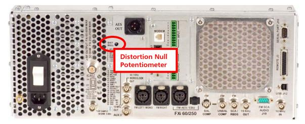
Figure 10 – Distortion Null Adjustment
