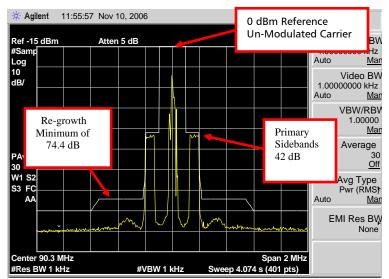
Figure 5 – Properly Aligned FM HD Radio™ Spectrum at -20dB
