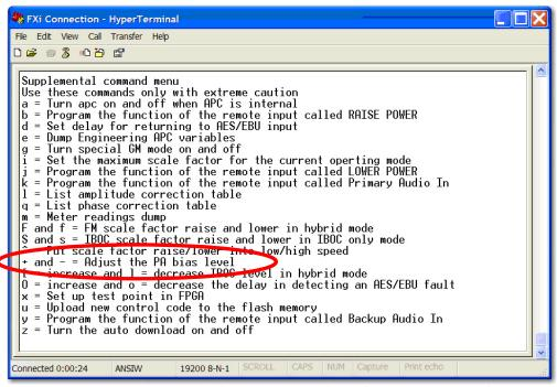
Figure 9 - "+" and "-" Command to Change Exciter PA bias
