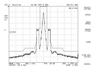
Figure 11 – Typical Properly Aligned FM+HD (-20dB Hybrid) Spectrum
