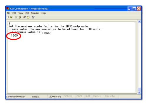
Figure 8 – "i" Command to Change Maximum Scale Factor
