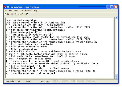
Figure 3 – HyperTerminal Supplemental Command Menu
