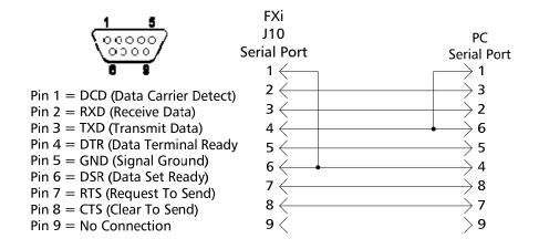
Figure 2 – Serial Cable / Null Modem Adapter Pinout
