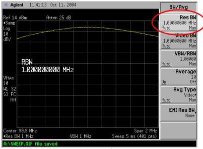
Figure 4 – Setting the top reference at 1MHz RBW.
